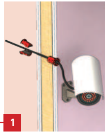
1 Single cable devices available for cable up to 14mm in diameter
